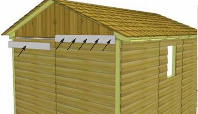
**54.** Attach **Rear Horizontal Gable Trims** to the back of the shed. Position over gable and wall seam with thick end of Bevel downward. Use **5 - 1 1/2" Finishing Nails** to secure each piece.
