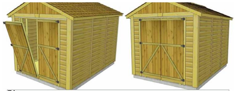
**71.** Position Left Side Door as per Step 70 and secure with 2" Black Screws. When satisfied with door positioning, complete all 2" Black Screw attachements. Note: Do not over tighten hinge screws when using screw gun. Tighten 3/4 of the way and use a Screw Driver to finish so as not to strip screws.
