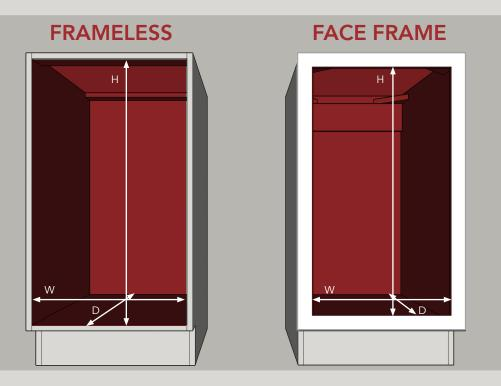
Rev-A-Shelf manufactures products that install into nearly all cabinet sizes. Make sure to correctly measure your cabinets to allow the best fit.
