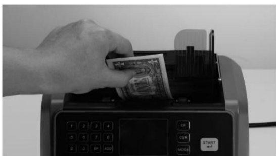
Feeding gap adjustment with one banknote
