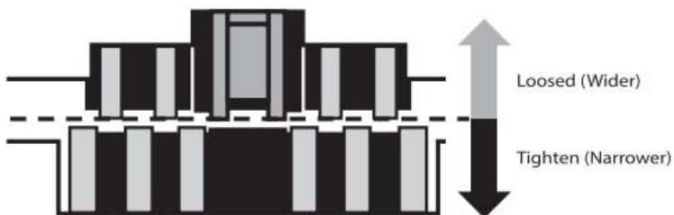
Feeding gap adjustment with one banknote
