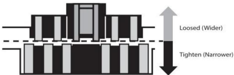
Feeding gap adjustment with one banknote
