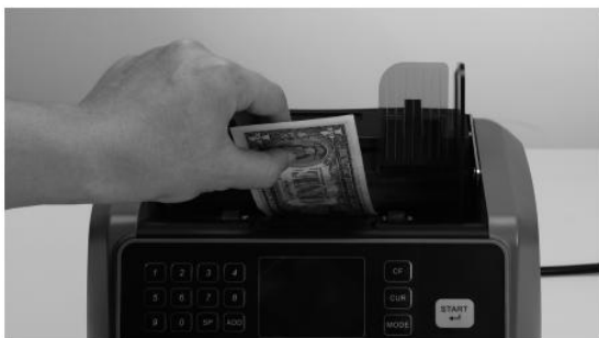
Feeding gap adjustment with one banknote
