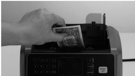
Feeding gap adjustment with one banknote
