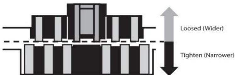
Feeding gap adjustment with one banknote
