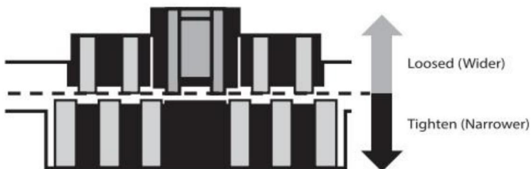
Feeding gap adjustment with one banknote
