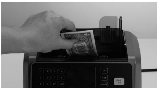
Feeding gap adjustment with one banknote
