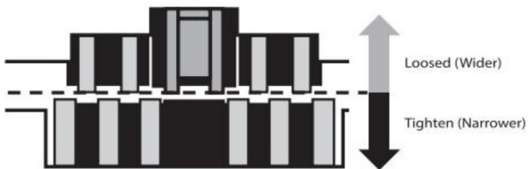
Feeding gap adjustment with one banknote
