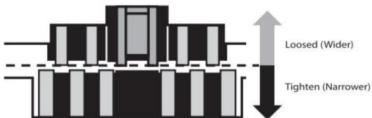
Feeding gap adjustment with one banknote
