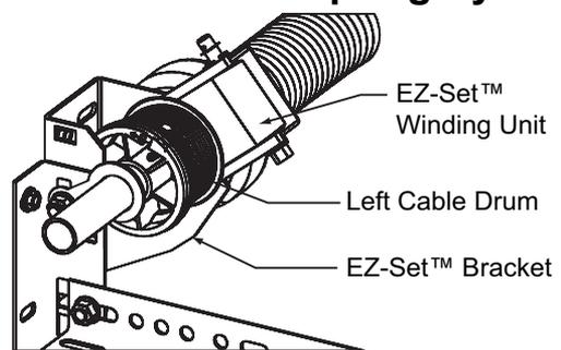
**NOTE:** The above illustration represents a composite of many of the features found on a variety of garage doors. While not representative of any one door, it provides a handy reference for the location of specific components
