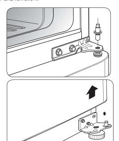
Loosen and remove the two bolts and use the Phillips head screwdriver to remove the Middle Hinge Bracket from the refrigerator housing. Set parts aside.
