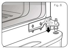
• Use the two bolts and the screw to refasten the middle hinge with the refrigerator housing. See Figure 9.
