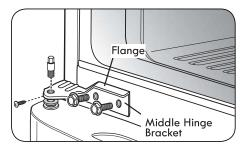
Insert the Decorative Screw into the outer hole on the right side of the housing. Attach cover on the right side. Cover is force-fitted.
