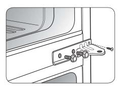
Remove the washer from the Bottom Hinge Pin. Using a 1/4" socket wrench, loosen and remove the Hinge Pin from the Bottom Hinge. Reattach the Hinge Pin to the opposite side of the hinge.
