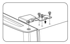
Slightly lift up the refrigerator door and remove it.
