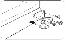
Remove the Decorative Caps on the bottom of the refrigerator housing. You will need these holes for the Bottom Hinge.
