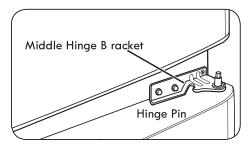
Turn the freezer door upside down on a non-scratch surface. Loosen the screw to remove the Door Closer/Stop and Hinge Pin Insert.
