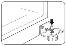
Using a 3/8" socket wrench with a 2-Inch extension and screwdriver, loosen the two bolts and one screw, and remove the Bottom Hinge from right side of the housing.
