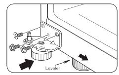
Turn the refrigerator door upside down on a nonscratching surface. Loosen the two screws to remove the Bottom Hinge Pin Insert Bracket with the Hinge Pin Insert.
