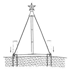
Outdoor: Affix the light show tree base frame to the ground using ground stakes.
