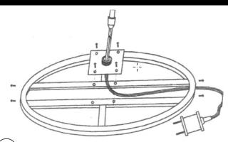
Affix the square metal plate to the base with the included bolts. Insert bolts at both sides of the base to secure the base. (Note: bolts used vary by model)
