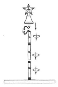
Screw the lower tube to the base. Then screw the next tube into the lower tube and repeat as needed. The power cord is pre-threaded through the tubes. Connect the star plug to the tube plug. Twist the plug ends to lock them together.
