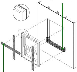
ZIP System tape or adhesive backed flashing (must meet AAMA 711 or AC148) sealed over window flanges. jambs
