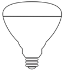
Philips-PAR30S Model # 477455 75W Equivalent/ 10.50W (2700K)
