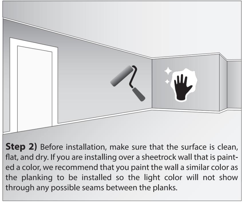
**Step 2)** Before installation, make sure that the surface is clean, flat, and dry. If you are installing over a sheetrock wall that is painted a color, we recommend that you paint the wall a similar color as the planking to be installed so the light color will not show through any possible seams between the planks.
