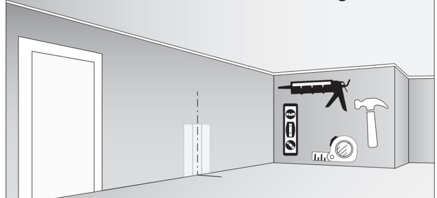
Start by finding the center of the wall and mark its location on the floor. Install the first plank on the wall centered on the mark with construction adhesive and nail in place with a brad gun (see instructions above). Use a level to make sure it is plumb. Next, attach planks on the left and right of first centered plank until you reach the corners of both walls. The width of the final plank at each corner will need to be trimmed to fit.
