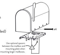
Once the mailbox is mounted, carefully push the plastic bracket up into the mailbox plate. Press the sides of the bracket inward making sure the four studs snap into the rectangular notches on the sides of the mounting plate as shown below.
