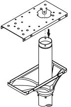
Install the assembled post into the ground. Ensure that the mounting plate is facing toward the street before installing into the ground.
