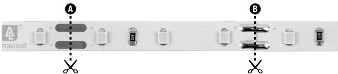
**IMPORTANT:** Always use the + / - indicators printed on the tape light to maintain the same polarity (+ to + and - to -).
