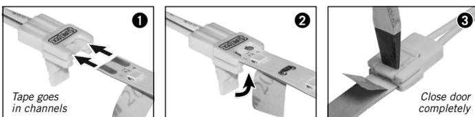
Splice connectors are used to join two strips, creating a continuous run of LED lighting.
