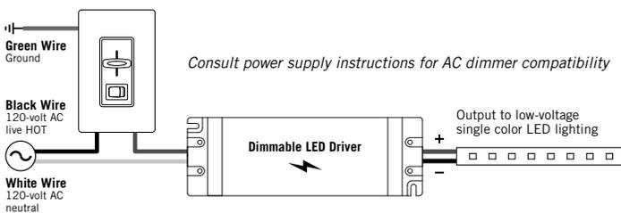
When using a 120-volt AC dimmer, the dimmable LED driver/power supply must be direct wired to household current.
