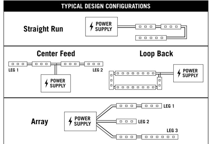
Choosing a higher wattage power supply does not necessarily mean you can run longer lengths of LED tape light. However, it will allow for more lighting legs in an array design. Exceeding the maximum lengths in the chart below will cause LEDs farthest from the power supply to appear dimmer when at 100% brightness due to voltage drop. Using a higher wattage power supply will not reduce the effect of voltage drop.
