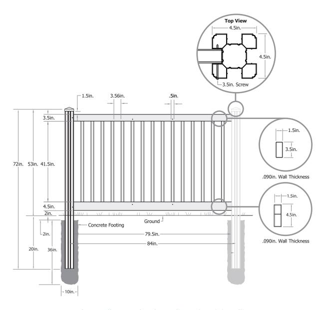
Please adhere to the above dimensions if installing around a pool to comply with BOCA code.
