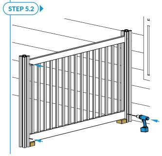
▶ Repeat in each remaining rail corner using (3) total 3½" self-drilling stainless steel screws.
