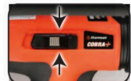
The Cobra+ Tool also features an adjustable power level for optimal penetration into the base material.
