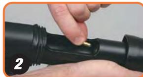
2 Insert a single load into the chamber with the rounded tip facing forward. Pull the barrel back to close the tool.
