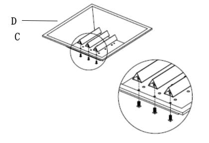
**5.**Turn completed base and slate top assembly right side up.Place Fire Bowl(D) into base as
