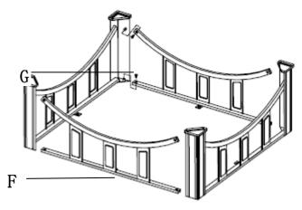
**4.** Put the assembled Leg(G)&F to the Slate Top(E), using M6 Nut(CC), then tighten all nuts by Wrench(DD).
