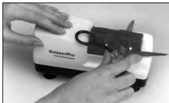
Figure 8. Start with the "Fine" Honing Stage.
