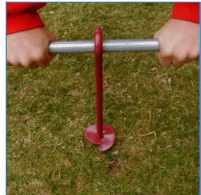
Note that your choice in Earth Anchor selection will depend on the type of soil that it is being installed in. For hard soils, often time with clay content, the smaller diameter helical screw Earth Anchors will likely provide the holding power required. For softer soils, the 6" diameter helical screw, 48" tall Earth Anchor may be required as you will need to install deeper in the earth to increase the anchor's holding power.
