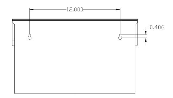
For wall mounts, use #8 or #10 pan head Phillips screws of adequate length to anchor the mailbox. For wood panel walls, screw length into the wall should be approximately 1". For masonry, stucco or metal walls, use a minimum #8 plastic anchor and screw.
