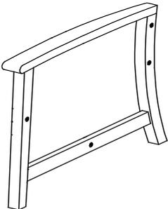
A wooden frame component similar to the right leg panel, but with the backrest rail curved in the opposite direction, with four circular holes for assembly. | Left Leg Panel (with<br>Leveler)  | 1   |
