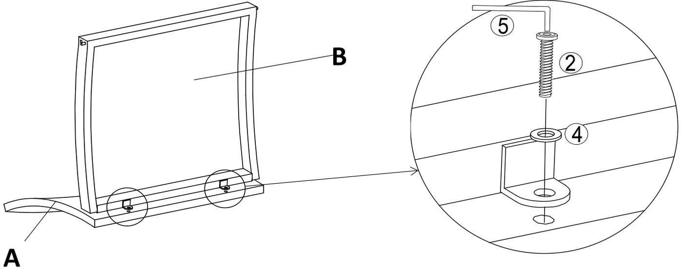
Lay down Backrest Panel (A) then attach Seat Panel (B) to Backrest Panel (A) by using Bolts (②), Flat Washer (④) and secure by Allen key (⑤).
