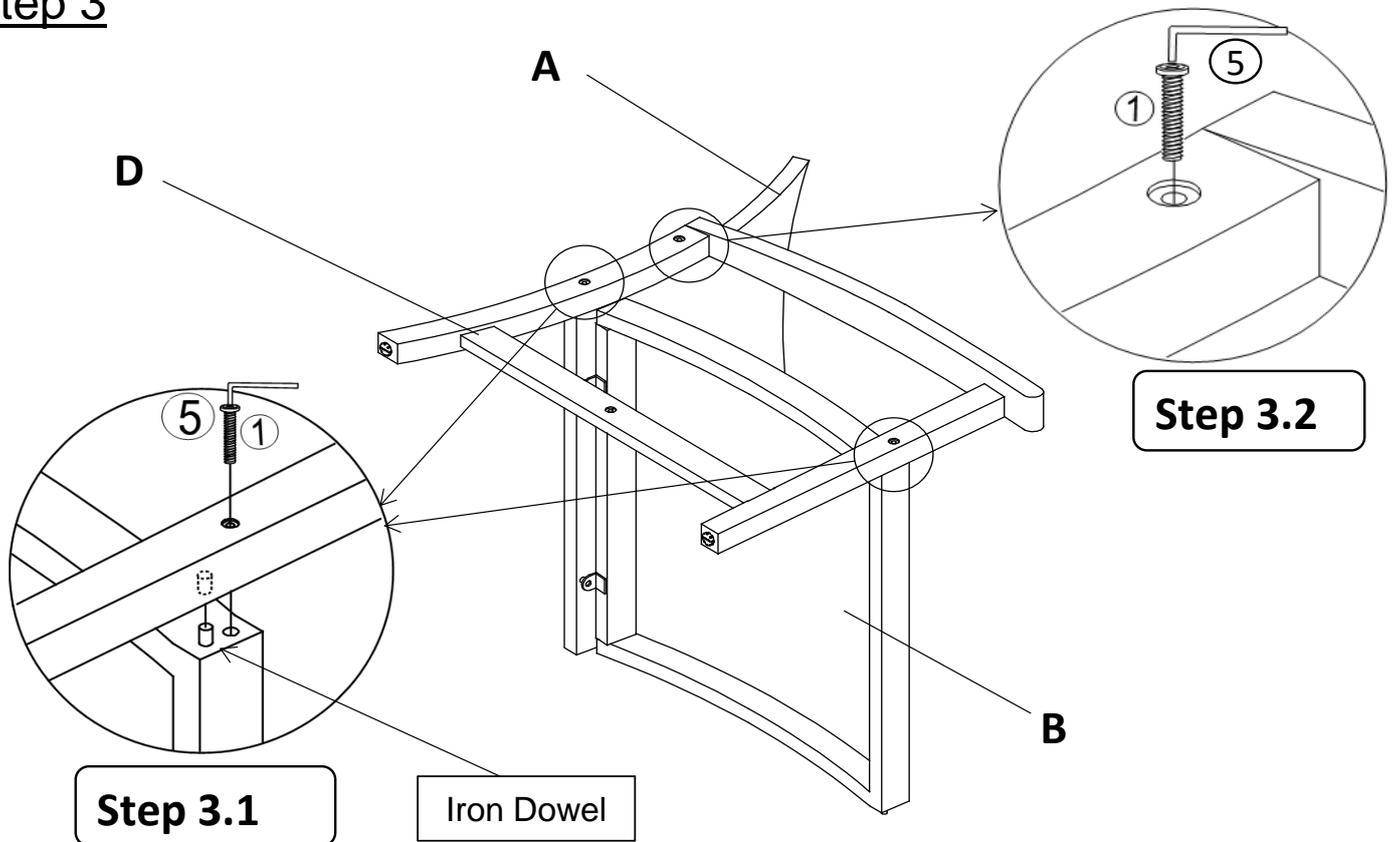
Position housing of Left Leg Panel (D) into pre-fixed iron dowel on Seat Panel (B) as picture above.
