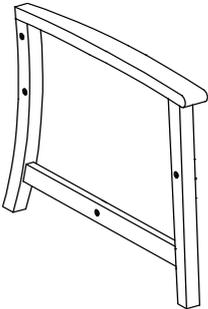
A wooden frame component consisting of a vertical leg, a horizontal seat rail, and a curved backrest rail, with four circular holes for assembly.             | Right Leg Panel<br>(with Leveler) | 1   |
