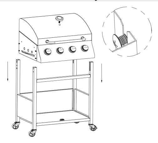
5. The body (1) is slided into the frame legs with 8 pcs pre-assembled M5 screws (See detailed pic.). Tight screws after body slided into position.
