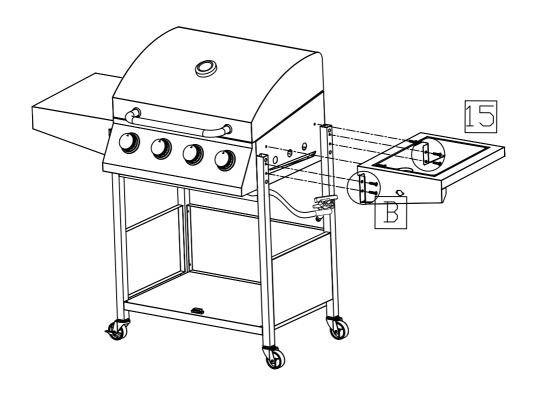
7. RH side shelf (14) is asssembled to the body with 6 pcs M5 screws (B).
