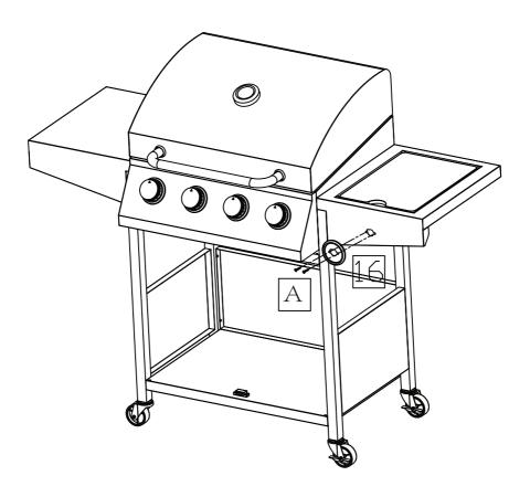
8. Side burner rotary switch base (16),side burner front plate and side burner valve (inside shelf front plate) are assembled together with 2pcs M4 countersunk screws (A).
