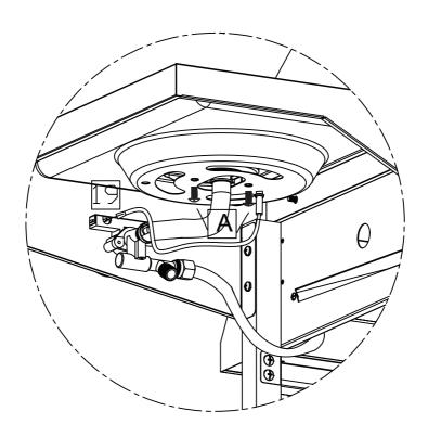
9-2. One end of ignition (19) is assembled to the side bunrer shelf with 1 pc M4 screw (A) and 1pc M4 nut (D). The other end is assembled to the valve connector.
