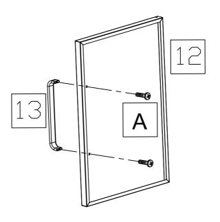
11. Handles (13) are assembled to front doors (12) with 4pcs M4 screws (A). Totally 2 pcs doors.
