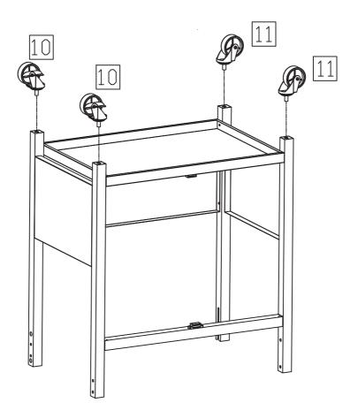
4. Assemble the 4pcs wheels (10&11) to the end of frame legs. Note: the 2pcs wheels with break (10) are always in the same side.
