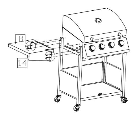
6. LH side shelf (14) is asssembled to the body with 6 pcs M5 screws (B).
