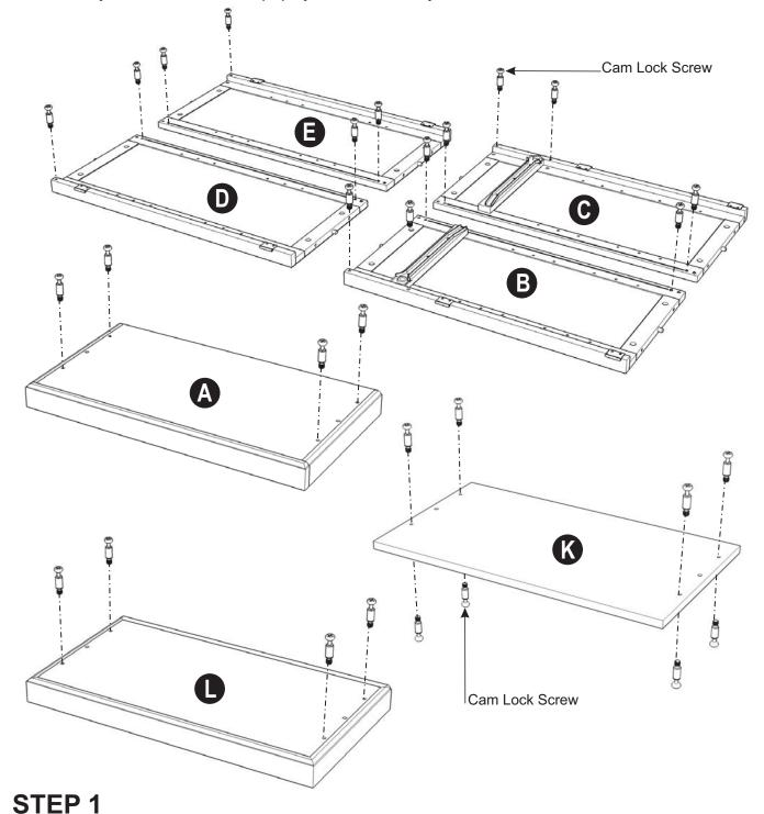
Put Cam Lock Screws into the pre-drilled holes of Top (A), (K) Side Panels (B),(C), (D), (E) Base (L) and tighten.
