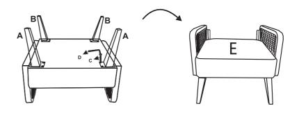
**STEP 2:** Use bolt C, allen key D to attach legs A to bottom of the seat E. Make sure all parts align then fasten all bolts to secure. And turn the chair base upright.
