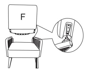
**STEP 4:** Align male and female metal bracket then insert backrest and push it all the way down to secure.
