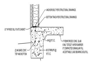
It is crucial to have a level foundation in place before starting the construction of the unit. A level foundation ensures the stability and proper alignment of the structure. If the foundation is not level, it can lead to issues with the unit's structural integrity and functionality, and shims may be required.
