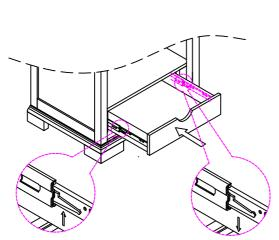
Pull the right clip upward and left clip downward at the same time, then draw the drawer box out.
