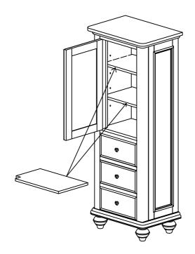
To adjust the shelf, please use a screwdriver to remove the 4 screw inserts and shelf support brackets which are under the shelf. Move the shelf and place the shelf support brackets into the pre-drilled holes. Then secure with screws.
