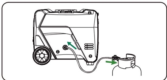
2. Fully open the Propane/LPG cylinder knob.
