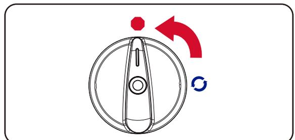
4. Turn cylinder valve to the OFF position.
