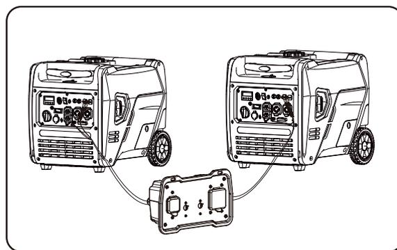
5. Start one of the generators and wait until the engine speed to stabilize.
