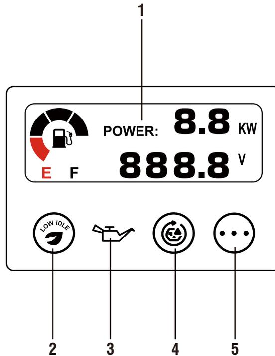
**1. LED Multi-Meter:** Displays voltage, power, fuel level, frequency, and running time.
