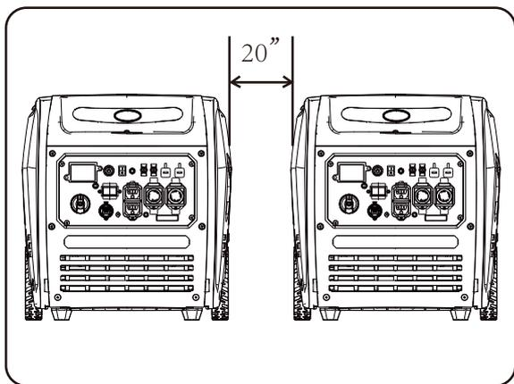
2. Both generators to be turned off and all electrical loads disconnected before paralleling operation.
