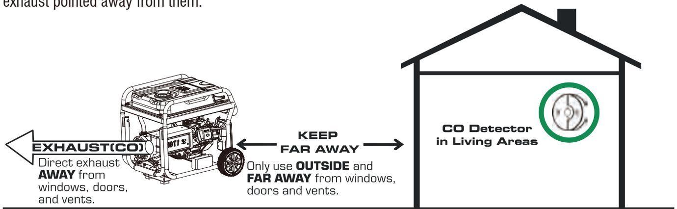
However, if the generator misused and operated in a location that results in the accumulation of CO inside an enclosed or partially enclosed space, CO WATCH- GUARD automatically shuts off the engine and notifies the user of what has happened and directs the user to read the instruction of CO WATCH-GUARD Action Label for steps to take.
