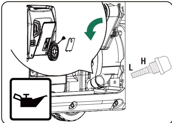
The engine is equipped with a low oil shut-off and will stop when the oil level in the crankcase falls below the threshold level.
