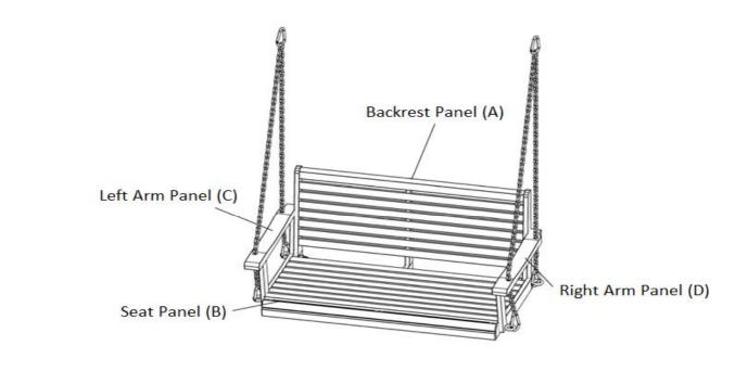
This Swing has multiple parts and may require up to 30 minutes to assemble. To give you an overview of the Swing, the above picture is to help you put the various parts into perspective. Please read through the instructions below to familiarise yourself with the parts and steps before assembly.
