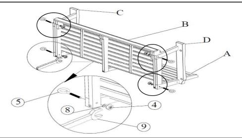
Insert the tenons of the Seat Panel(B) into the mortises of Left Arm Panel(C) and Right Arm Panel(D), then attach using Lock Nuts(4), Washers(8), and Eye Bolts(5), with Wrench(9) as shown above.
