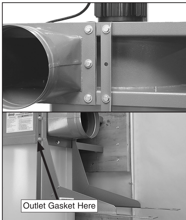
Figure 18. Model G0441 outlet port and filter L-braces installed.
