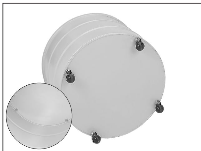
Figure 24. Casters attached to the lower collection drum.
