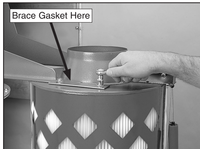
Figure 19. Mounting filters to the braces.
