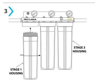
Inspect the O-Ring on the housing for any damage or cracks. Ensure the O-Ring is sitting properly in the groove. Lubricate the O-Ring and housing threads with silicone lubricant or a food-grade lubricant.
