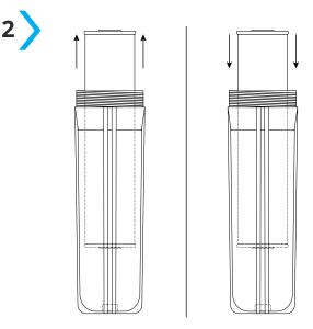
Remove the old filter and install the new filter. Ensure to center the filter cartridge properly in the housing.
