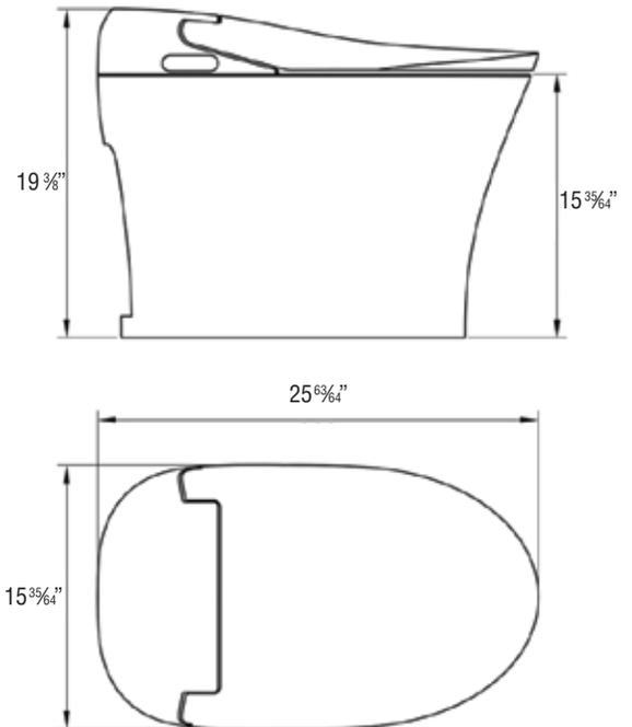
This toilet is designed to rough-in at a minimum dimension of (12") from finished wall to C/L of outlet. Supply not included with fixture and must be ordered separately.
