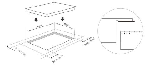
2. It is essential that the Radiant Cooktop is well ventilated and that the air intake and exit are not blocked.
