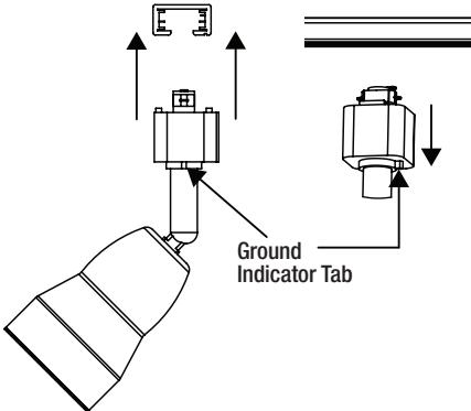
**CAUTION:** Adapter is designed to lock into the track section by turning adapter in one direction only. Turn the "ground indicator" tab towards the "ground groove" on the track to align the ground tab with the ground conductor inside the track.
