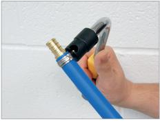
2. Twist the nub with the tool until the clamp breaks or loosens.
