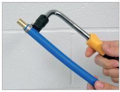
1. Slide the pinch clamp nub into the removal tool slot. If the nub is too large to fit into the tool, use the clamp tool to pinch the clamp one more time.
