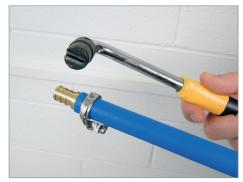
3. Remove the tool from the clamp, then remove the clamp from the pipe.
