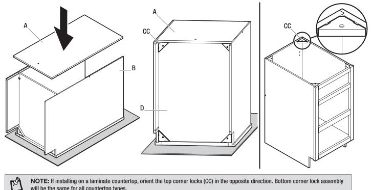
NOTE: If installing on a laminate countertop, orient the top corner locks (CC) in the opposite direction. Bottom corner lock assembly will be the same for all countertop types.
