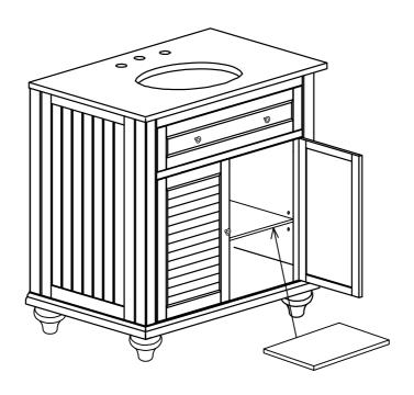
To adjust the shelf, please use a screwdriver to remove the 4 screw inserts and shelf support brackets which are under the shelf. Move the shelf and place the support bracket into the pre-drilled insert holes. Then secure with screw inserts.
