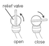
So, every time you start the pump, open the relief valve and exhaust the [air/water] stream for about 15 seconds (or more, depending on when the air/water stream becomes pure water stream). Then close the valve and start misting.
