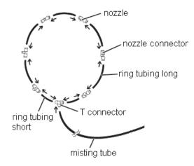
You can now put the ring onto an outdoor fan. Use the cable tie to tie the ring to the fan's front mesh. Fan can use the power socket provided by the pump unit or any other appropriate wall socket.
