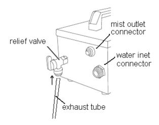
**TIPS!** The pump tubing will always catch air when pump starts drawing water in. Air being sucked into the tubing will quickly form bubbles. When bubbles are big enough, it will block the water flow inside the tubes or reduce the pump pressure, thus weakening the misting effect.
