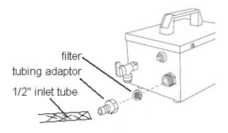
The other end of the 1/2" tube can be set free into a water tank or it can be connected directly to a water faucet. Faucet adaptor is not included.
