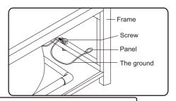
The bathtub must be connected to the ground. Power outlet must be sealed well.
