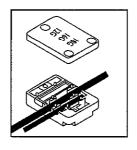
Take the end of the wire that is attached to the fixture and press it firmly into the channel marked 18G.
