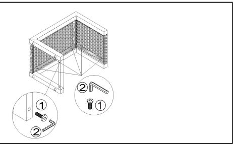
Align Side Support Bar(A) to Side Panel(C), Top Panel(B), and Base Support Bar(D).
