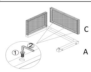
Attach Side Panel(C) to Side Support Bar(A) using Bolts( $\bigcirc$ ) with Allen Key( $\bigcirc$ ) as shown above.
