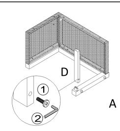
Attach Base Support Bar(D) to Side Support Bar(A) using Bolt(1) with Allen Key(2) as shown above.
