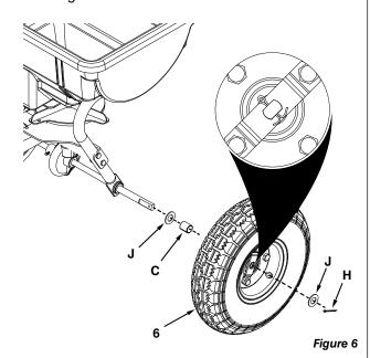
STEP 7 (SEE FIGURE 7): Attach the other wheel by sliding onto the right end of the axle a washer (J), a spacer (C), a wheel (5), and another washer. Secure with a cotter pin (H) by sliding it through the hole in the axle and bending the ends.
