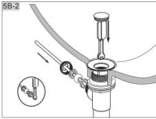
As shown. Place the Drain stopper into the drain body from the top rear. Slide the ball rod into the Ball Rod Opening through Stopper Hole, and threaded it on to the Drain Body.
