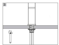
If necessary, tighten screws using a adjustable wrench until the faucet is firmly connected to the sink.
