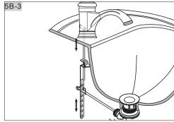
Insert Lift Rod through Lift Rod strap and secure with Set Screw. Place the Ball Rod through one of the holes on the Lift Rod Strap. Secure it with the Spring Clip. Adjust the height of the lift by resetting Set Screw. No interference between faucet and knob.
