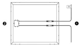
Connect the bare wire end of the positive cable 4 to the "SOLAR +" input of the charge controller 1. Connect the negative bare end to the "SOLAR -" input. Now, you can mount the GS-PWM-20A charge controller to an indoor wall or within a NEMA-3R rated enclosure.
