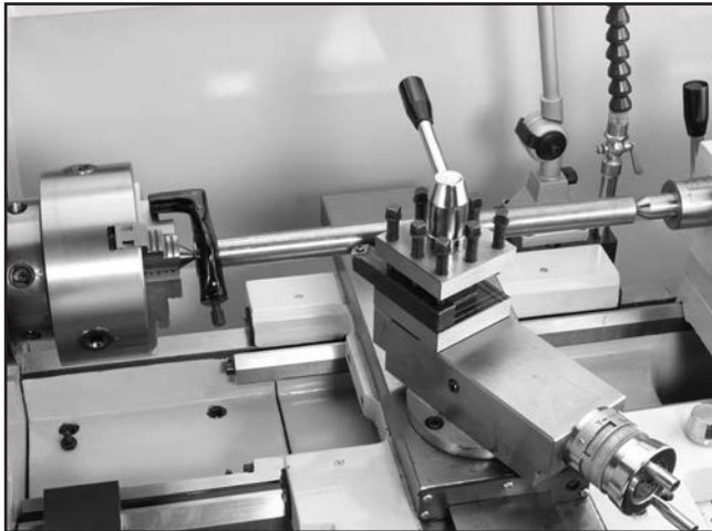
Figure 33. Example of stock mounted between the centers.
