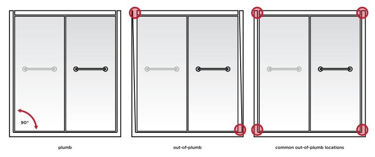
Most Delta Shower Doors are designed to accommodate out-of-plumb conditions up to 3/8". If your shower door environment is out-of-plumb, simply rotate adjustment bushing to lower or raise the glass.
