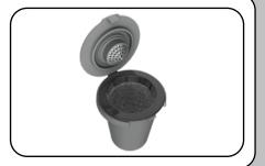
Remove the capsule chamber from the brew head and insert reusable filter cup.
