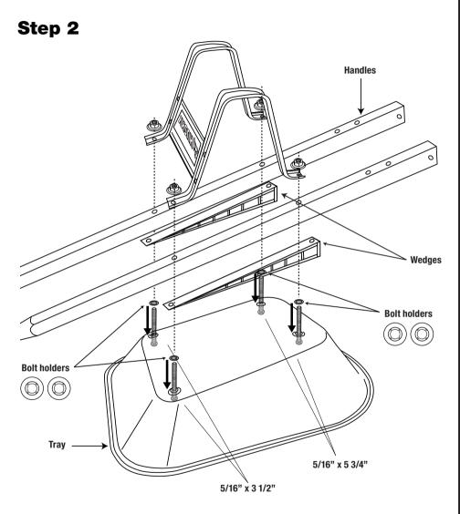
Insert the screws, fix them with a bolt holder to keep them in place up to the top. Once the screws are fixed, turn the tray upside down and set the steel handles and then the legs assembly.
