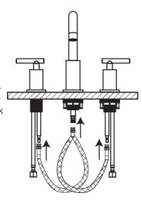
Note: The black water hose must be installed crosswise, as shown in the figure.
