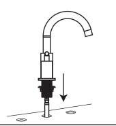
5. Carefully screw the male ends of the cold and hot water supply hoses into the respective faucets (blue=cold, red=hot) and tighten firmly by hand.
