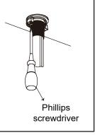
**6.** Fit the handles onto the sink using the correct outside mount holes and apply steps #3-#5 above to secure the handles.
