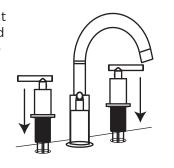
**9.** Connect the hot and cold water hoses to the water supply valves. Secure the connections with a wrench. Open water supply valves and check for leaks.
