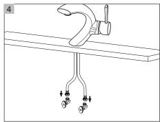
Connect hot and cold water supply lines to the Water Supply Valves.
