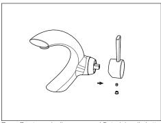
Turn off water and relieve pressure! Detach handle button using a small flathead screwdriver, unscrew set screw using Allen Wrench and take off handle.
