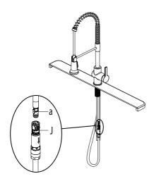
Push the quick connector (J) firmly upward and attach it to the receiving block (a). Pull down moderately to ensure the connection has been made.
