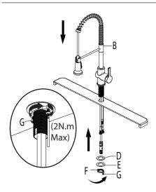
Shut off the water supply. Place faucet (B) through the hole in countertop. Secure the faucet (B) to the countertop using the rubber washer (D), metal washer (E) and mounting nut (F) provided. Tighten screws (G).
