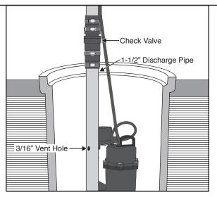
2. Measure, cut and install discharge fittings, check valve, and piping. Drill a 3/16" hole in the discharge pipe, level with the top of the pump.
