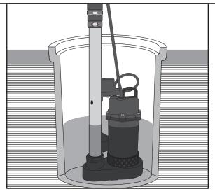
4. Test operation by adding water until float rises, pump turns on, and the water level drops. Float will lower with the water level and turn the pump off.
