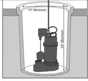
Ensure basin is clear of all debris and place pump on hard level surface (not dirt or gravel). 14" x 24" minimum basin size required.
