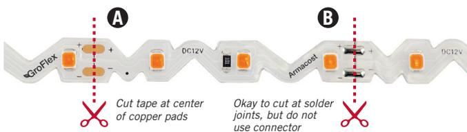
**IMPORTANT:** Always use the + / – indicators printed on the tape light to maintain the same polarity (+ to + and – to –).
