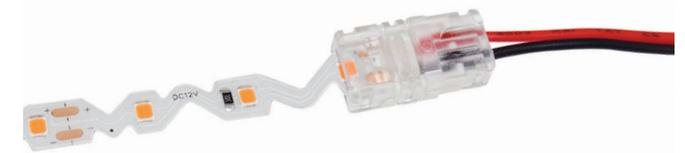
Use one WireGrip in combination with the factory-soldered wire leads, or use two WireGrip connectors, connect one on each end of the tape. Measure the gap and cut a length of wire to span this distance. 22 to 18 gauge wire is generally recommended. Do not coil excess wire; shorter lengths and thicker wire will mean less voltage drop and higher brightness.
