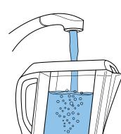
Once pitcher is attached to the filtration dock, it will automatically begin filtering. There will be a 5-10 second delay before the outer reservoir starts to fill.
